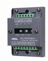
SB-LED650MA is the 3 channels LED Driver with DMX512, interface. Constant voltage with PWM output for dimming, RGB LED strip for changing color.
