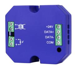
SB-IR-EM is the IR code sending device, and 200 infrared codes can be stored in it. By using the HDL IR learner (another device) to learn the IR codes from the normal remote, and downloaded into this device. The software can program and use the IR codes to control the IR device, such as TV, DVD, AC, Amplifier, etc.
