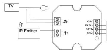
Note: Take TV as an example. Connect the power supply cable to the current detection port, when turn on or turn off the TV, the system will detect the status. And the system will read the current when turn on or turn off the TV. Use the average current of the two values and write it down in the software, "The standby current threshold", after setting, the system will know the power status of the TV.
